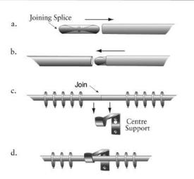
For poles over 200cm Slide the joining splice into the first pole end(a). Then push the poles together(b). Slide on your rings remembering to leave one at each end as an end stop(c).
