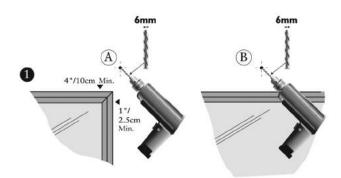
Mark & drill top holes of the support (A) using a 6mm drill bit. On longer length poles mark and drill top hole (B) in the middle for centre support. Fix screw until screw head is approx. 3mm from the wall.
