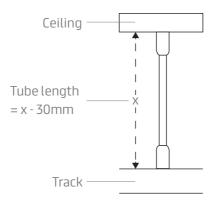
8. For suspension rods refer to figure above. Each bend must be supported by a 313 hanger (see figure below) assembly no further than 350mm from either leg of the bend.
